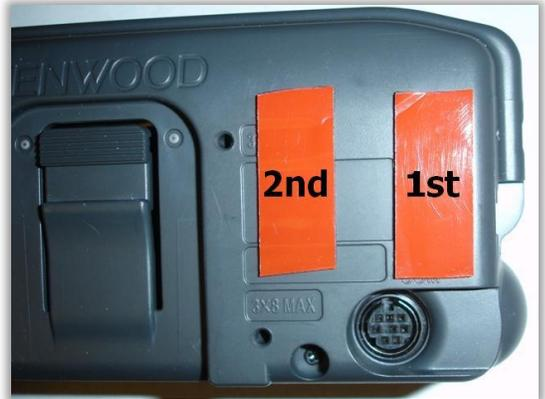
Figure 1: Tape Size and Placement
